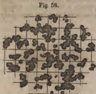
Fig. 58. Microscopic appearance of sublimed sulphur. (The micrometer squares are equal to those seen in Figs. 59 and 60.)
